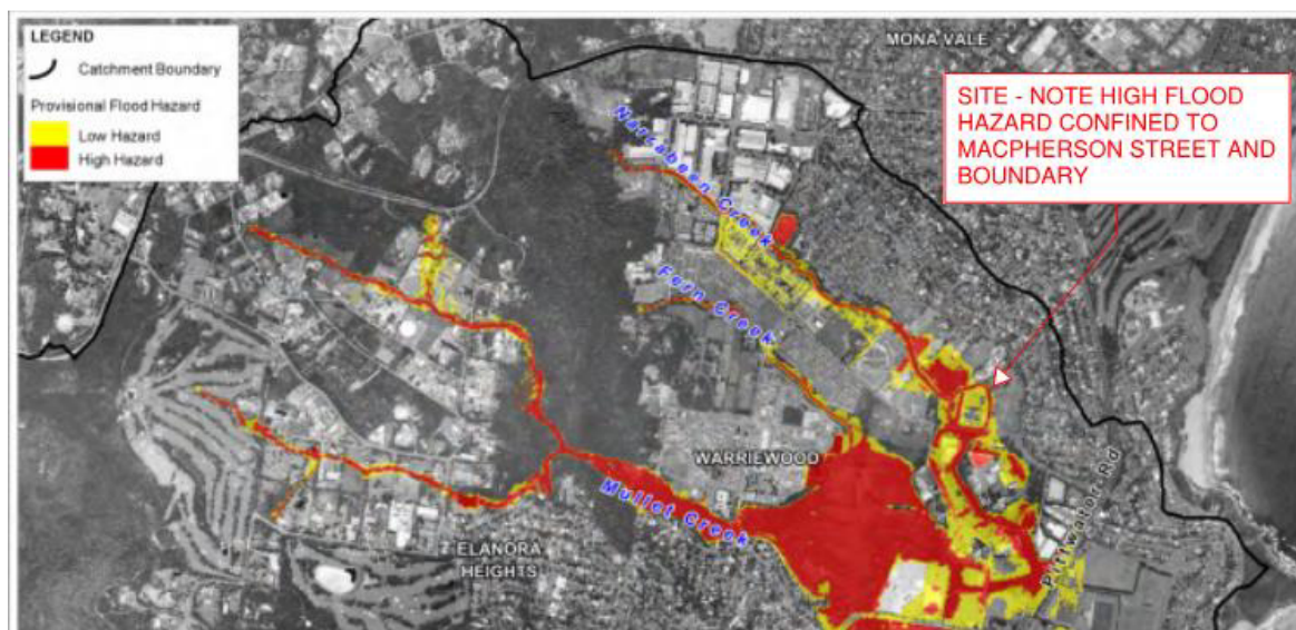
Figure 2: Flood Hazard Extract (From Narrabeen Lagoon Flood Study,[Map A28] BMT WBM 2013)
